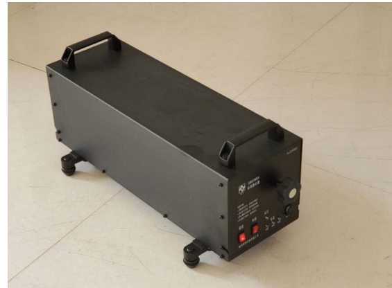
Fig. 4. Tapping machine for the impact sound insulation measurements.
