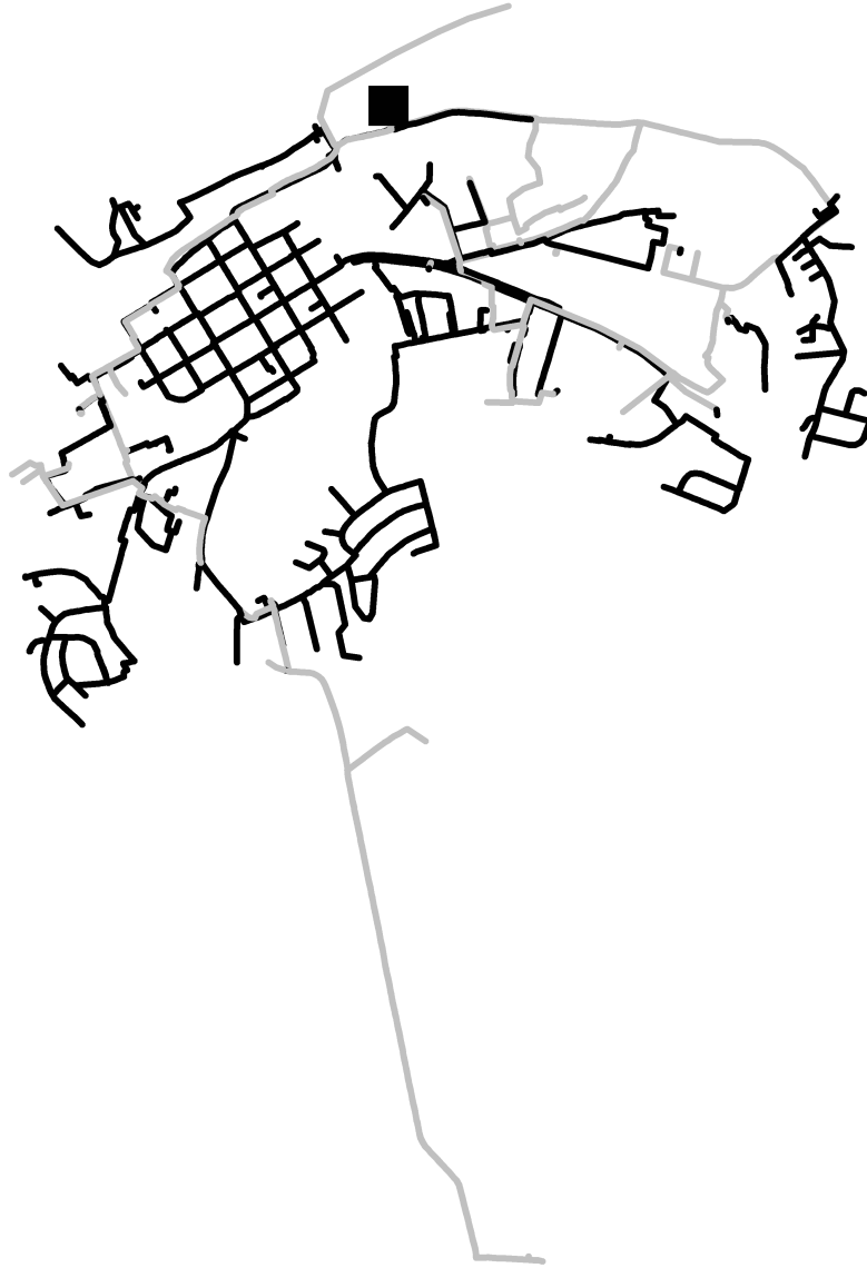
Figure 6: Structure of the gas distribution network in Chełmno, grey lines – medium pressure pipes, black lines – low pressure pipes [27].
