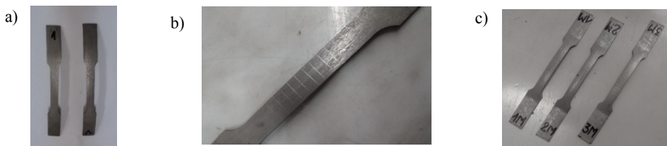
Fig. 5. Test samples a) after milling, b) after tracking, c) with flattened ends
