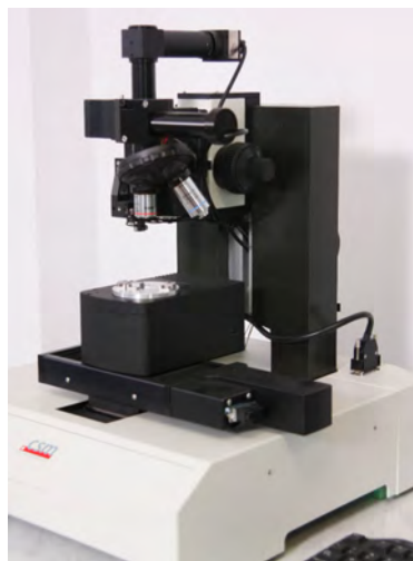
Fig. 2. The view of Nanotribometer used in the research
