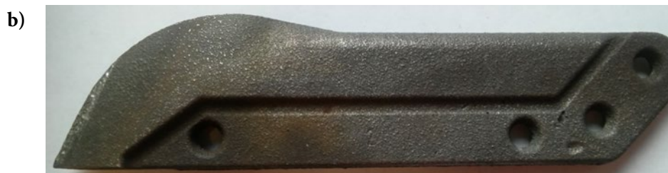
Fig. 11.2. Laser alloyed coulters flap after wear test
