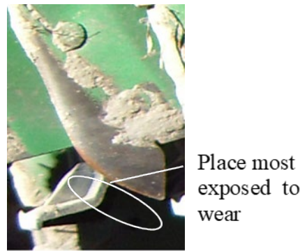
Fig. 2. Coultter flap fixed in agriculture machine with place most exposed to wear marked.
