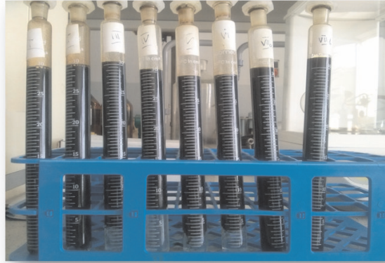
Fig. 2. Amount of separate water from oil modified after 1 hour at a temperature of 20°C
