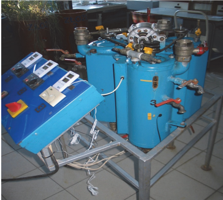
Fig. 1. Laboratory scale research installation for anaerobic sewage sludge digestion (source: W. Dąbrowski)
