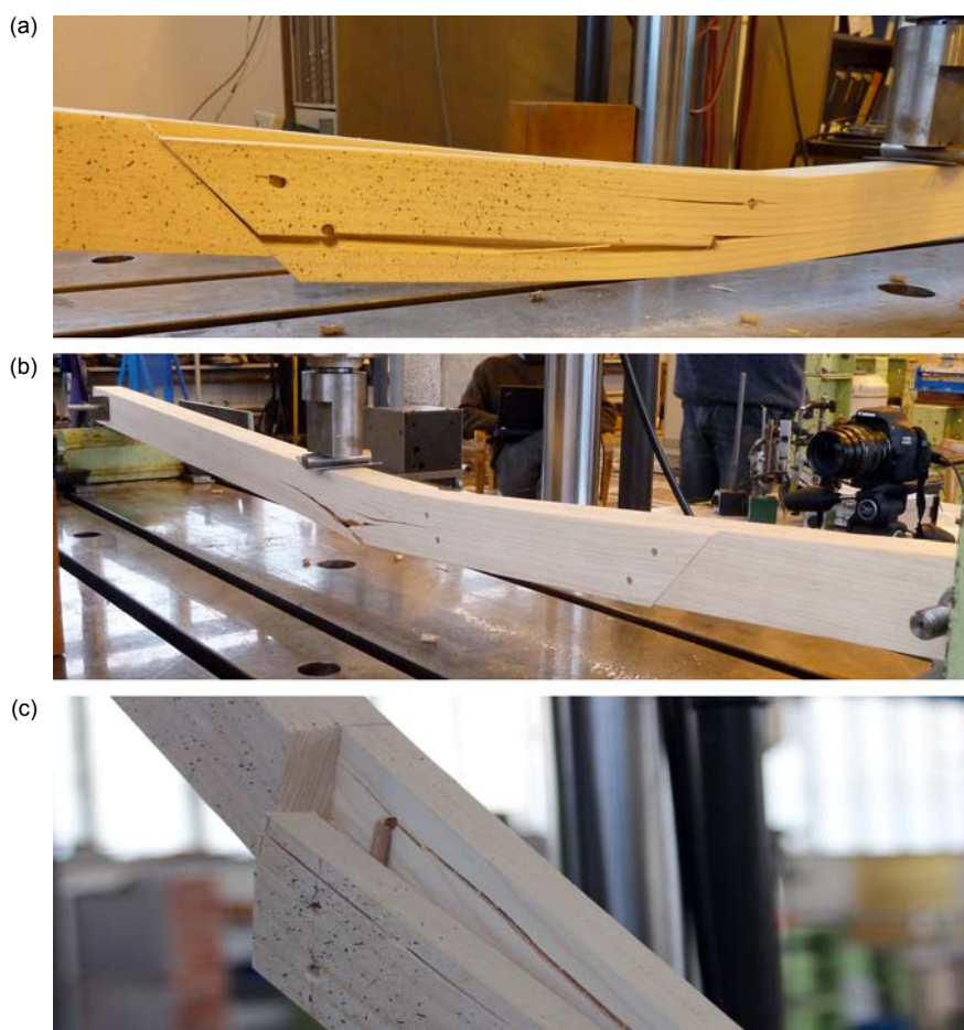
Fig. 4. Common failure patterns (a), (b), and (c)
