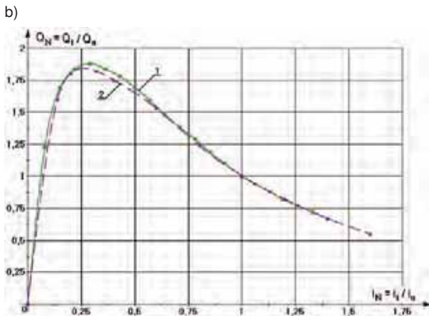
Fig. 3. Dependencies of the normalized quantity of luminous energy produced by TLS and SLS within ADG in the process of regulation of a luminous flux: a) TLS: 1 – HL 42 = 35 W; 2 – HL XENON 42 = 60 W; 3 – HL 28 = 35 W; 4 – IL PILA 60 W; b) SLS: 1 – luminarie with 42 LED total power 15.5 W; 2 – PARATHOM CLASSIC GLOBE 10.5 W
