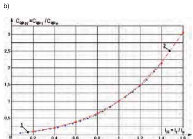
Fig. 4. Dependencies of the energy efficiency of the luminous flux regulation from the standpoint of the normalized specific cost of unit of luminous energy produced by LS within ADG: a) TLS: 1 – HL XENON 42 = 60 W; 2 – IL PILA 60 W; 3 – HL 42 = 55 W; 4 – HL 28 = 35 W; b) SLS: 1 – luminarie with 42 LEDs DURIS E5 of the total power 15.5 W; 2 – PARATHOM CLASSIC GLOBE 10.5 W
