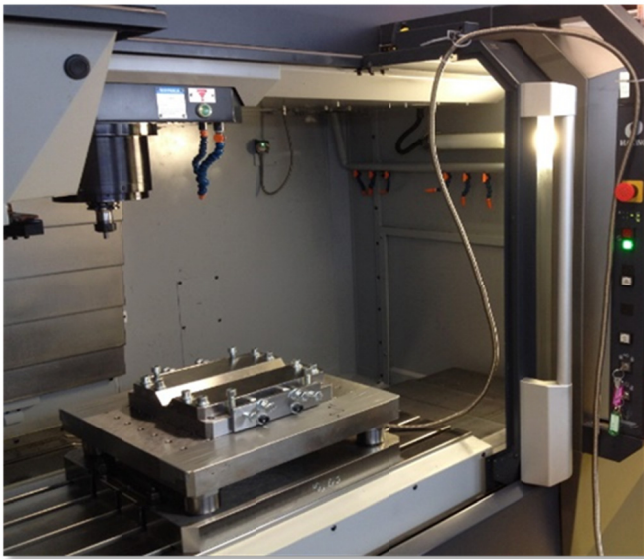
Fig. 3. View of 3 – axis CNC milling machine adopted for realizing FSW process
