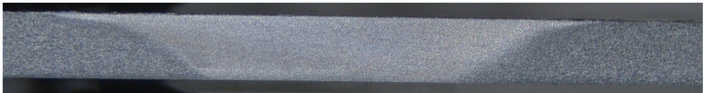
Fig. 9. Transverse view of a weld made with a carbide tool WT1 joint of AA 2024 T3 sheet of 1 mm thickness using carbide tool with smooth shoulder at 2000 rpm and welding speed 200 mm/min (No. 2)
