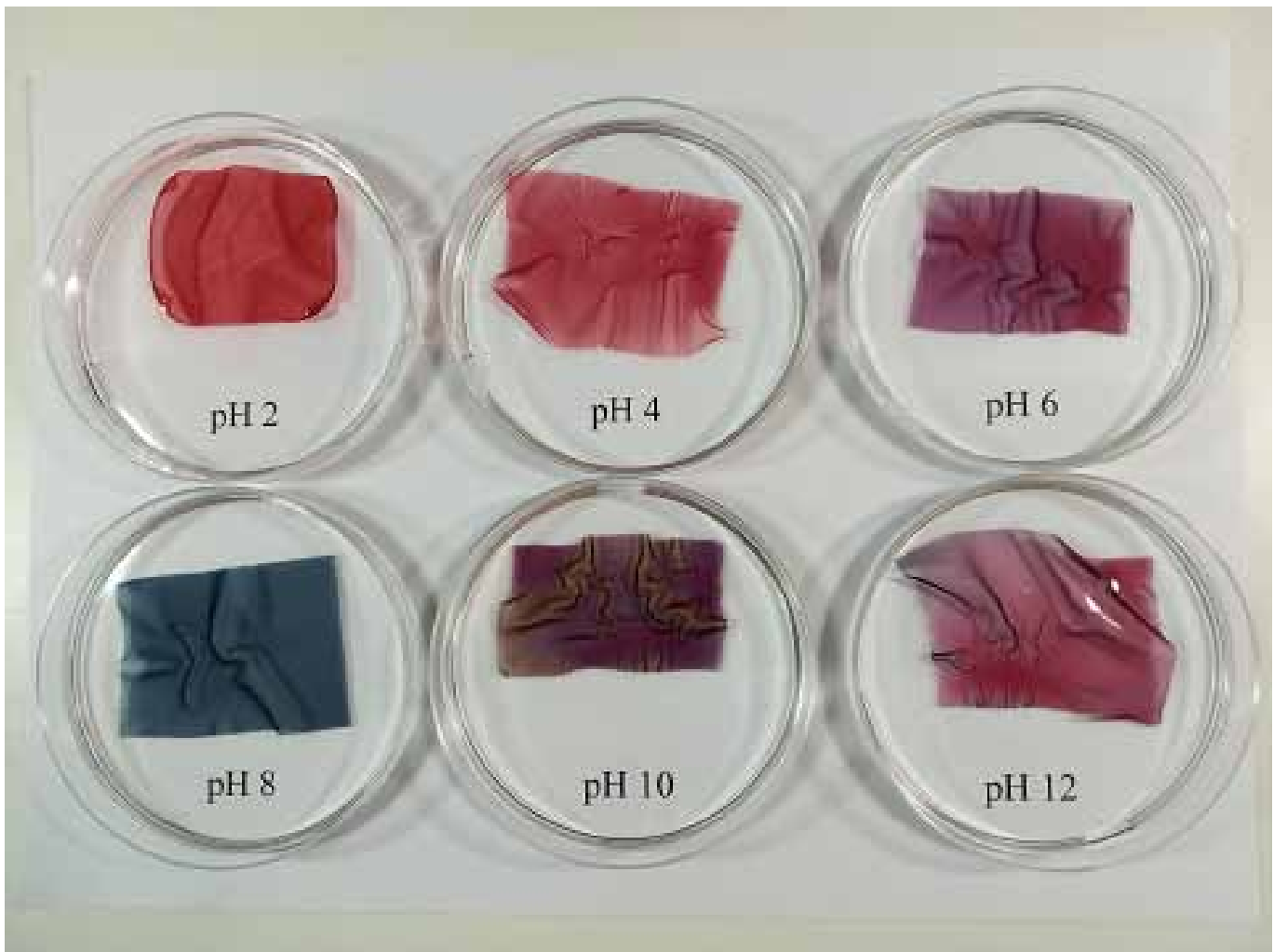
Fig. 4. Reaction to the changing pH from 2 to 12 for films prepared with the infusions of blackcurrant pomace (AS1,5%_CP5%).
