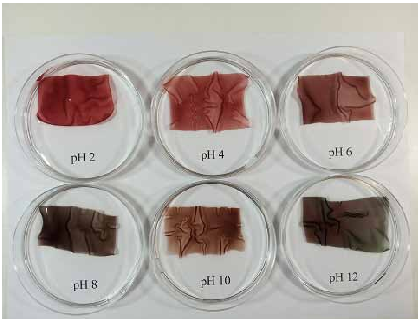
Fig. 3. Reaction to the changing pH from 2 to 12 for films prepared with the infusions of chokeberry pomace (AS1,5%_A5%).
