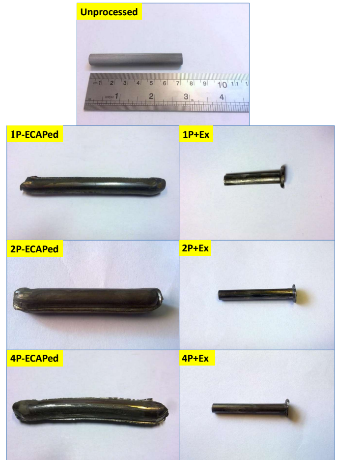
Fig. 3. Unprocessed, ECAPed and extruded samples illustration
