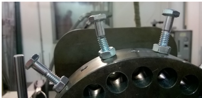
Fig. 7. Bolt #9 notched and bent in the forward direction
