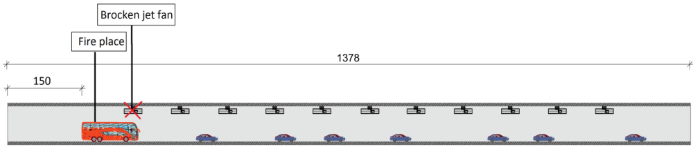
Fig. 4. Fire place in tunnel
