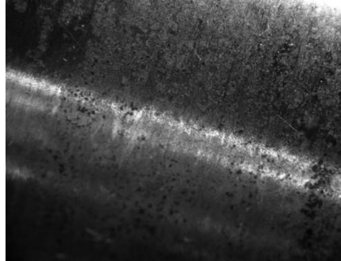
Fig. 6. Raceway of the main shaft of fuel injection pump
