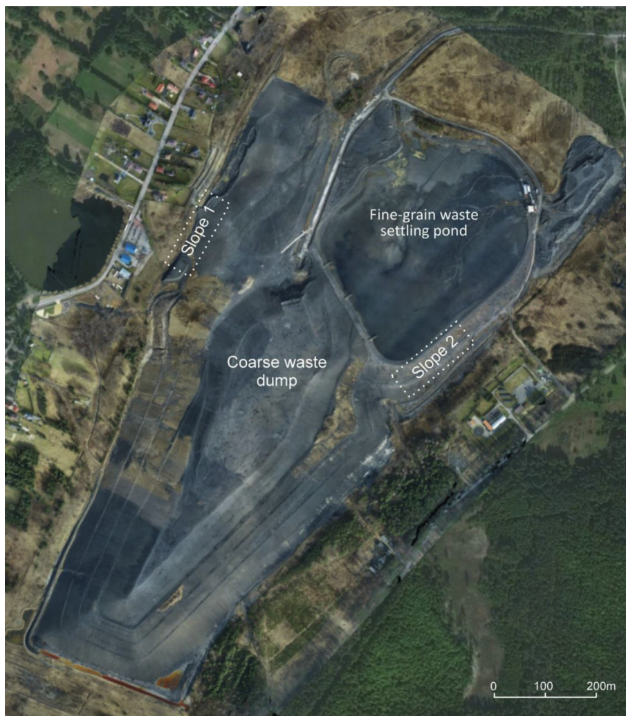
Fig. 1. The ZG Janina TAURON Wydobycie S.A. dumping ground in Libiąż and localization of analyzed slopes.
