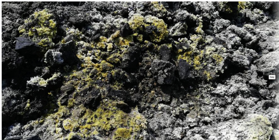
Fig. 8. Efflorescences of sulphur (yellow) and salammoniac (white) on the surface of Slope 1 in Zone 2.
