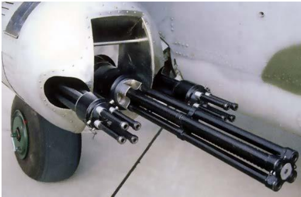
Figure 2. One JakB-12.7 and two GSchG-7.62 in universal helicopter nacelle (UHN)
