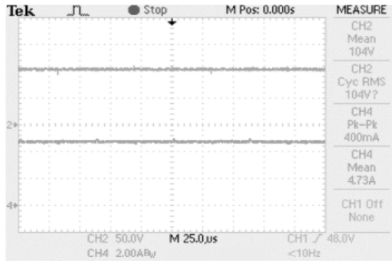
Fig. 9. Output voltage and load current waveforms for 16 kHz
