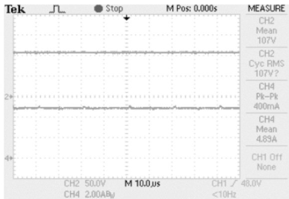
Fig. 11. Output voltage and load current waveforms for 50 kHz
