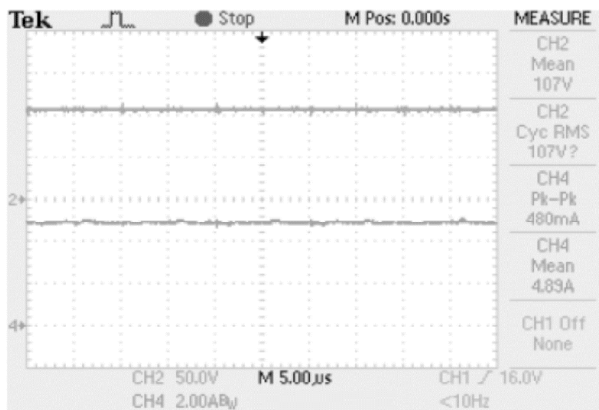
Fig. 13. Output voltage and load current waveforms for 100 kHz
