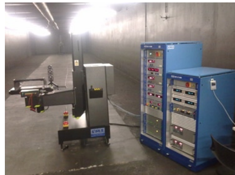
Fig. 4. Measurement tunnel for photometric study of various type of car lamps
