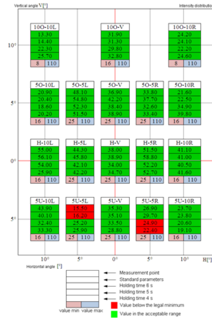
Fig. 8. Impact of changes in mould holding time on the intensity of light emitted by lamp
