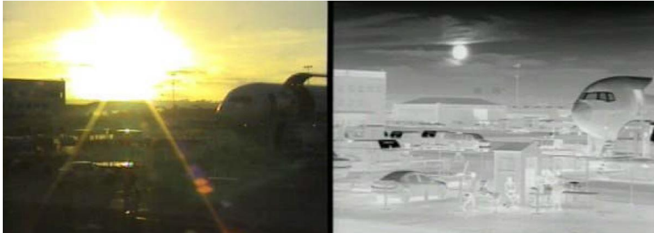
Fig. 1. An example of glaring effect of sunlight on an image recorded with a camera working in the human vision range (right) and in the infrared range (left) [ http://www.tcs.es/component/tags/tag/camaras-de-seguridad.html?start=20 (access 12.05.2016)]
