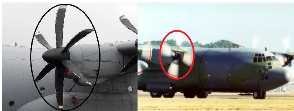
Fig. 6. Observation of a revolving propeller at different angles
