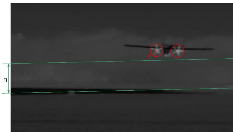
Fig. 11. Determining plane altitude over aerodrome — range 250 m
