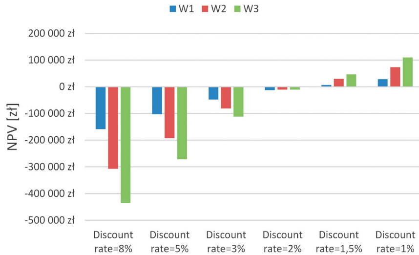
Fig. 16. NPV ratio for the considered PV plant options with various discount rates
