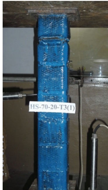
Fig. 12. Failure mode of column HS-70-20-T3(1)
