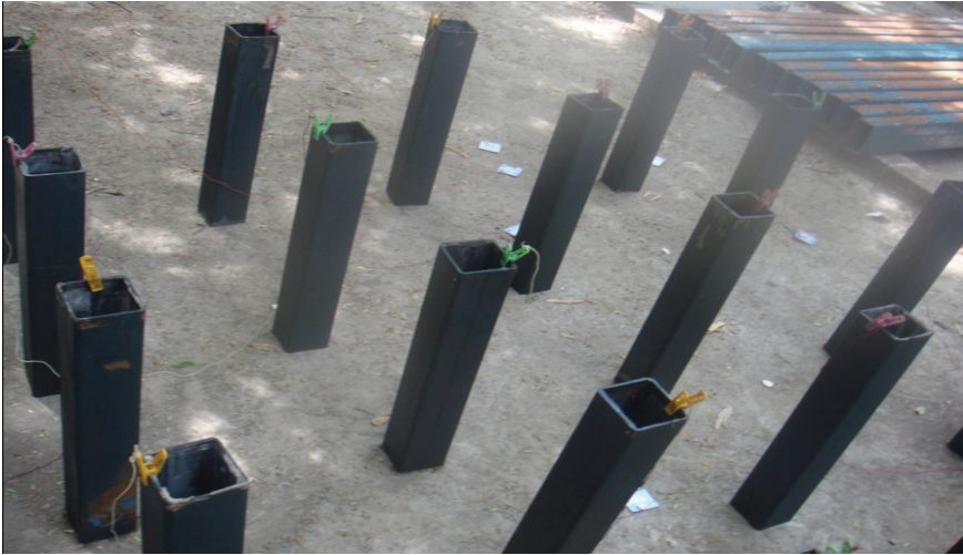
Fig. 2. Specimens before corrosion
