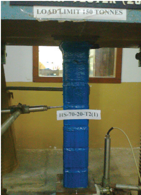
Fig. 11. Failure mode of column HS-70-20-T2(1)
