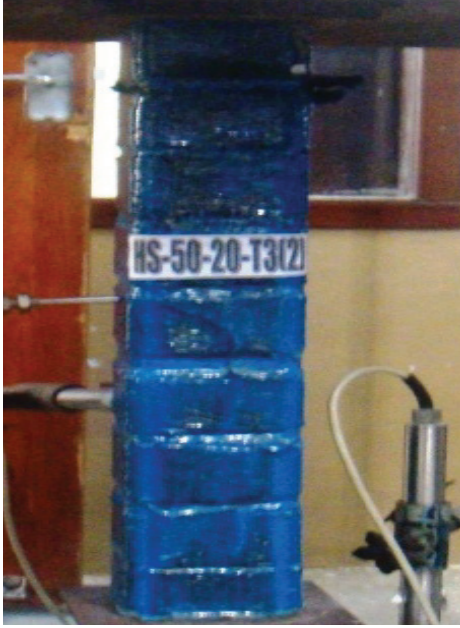
Fig. 9. Failure mode of column HS-50-20-T3(2)
