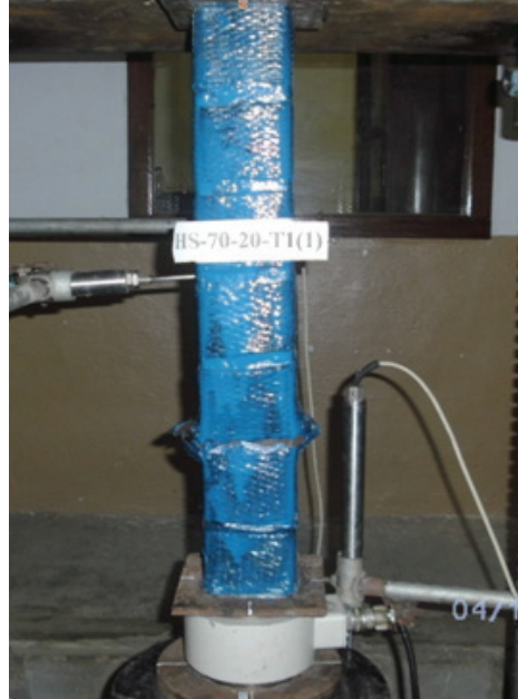
Fig. 10. Failure mode of column HS-70-20-T1(1)
