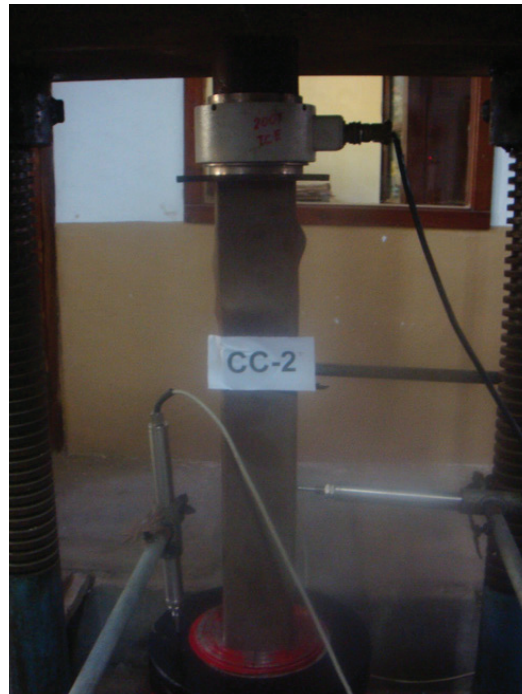
Fig. 6. Failure mode of column CC2
