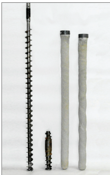
Fig. 8. Pictures of auger models which were used for pile installation and pile models after removal from the soil (starting from left: CFA auger; SDP auger; CFA pile model; SDP pile model)
