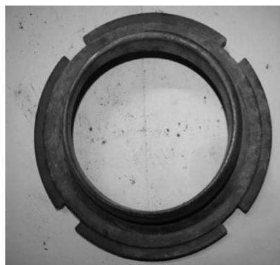
Fig. 8. Macroscopic image of the directional sleeve after operation in the crusher
