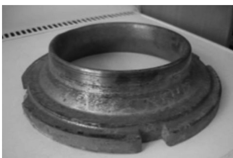
Fig. 2. Macroscopic image of the tested directional sleeve (feed inlet) of the SANDVIK CV117 centrifugal crusher
