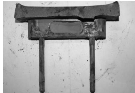
Fig. 14. Macroscopic image of the rotor tip cladding after operating in a crusher
