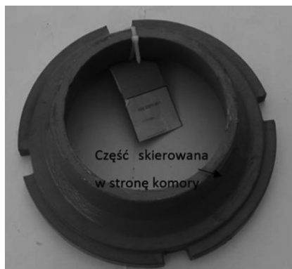
Fig. 7. Macroscopic image of the directional sleeve prior to operation in the crusher
