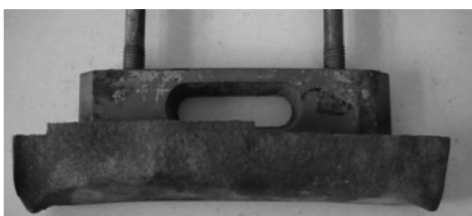
Fig. 4. Macroscopic image of the tested lining of the rotor ends in the SANDVIK CV117 centrifugal crusher
