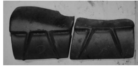
Fig. 12. Macroscopic image of the rotor hammer assembly after operating in a crusher
