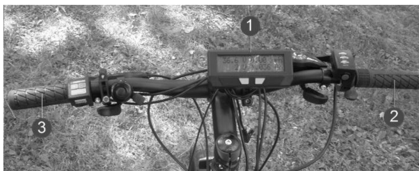
Fig. 2. General view of the electric bicycle handlebar: 1 – board computer; 2 – right handle; 3 – left handle
