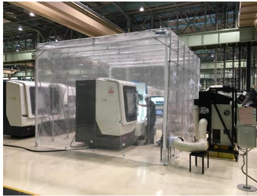
Fig. 10. Portable temperature variable booth and air conditioner
