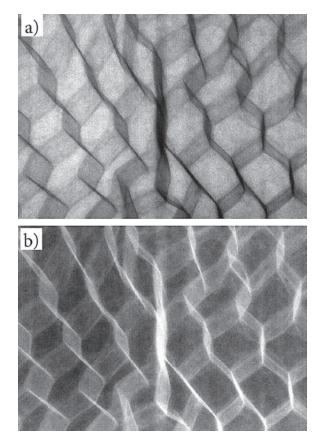
Fig. 9. Digital image of honeycomb structure airplane wing fragment get with digital solid-state transducer S10811-11: a – positive; b – negative
