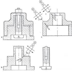
**Fig. 7.** Test bench for bolts of nuclear reactors: (a) total view; (b) plunger; (c) body; (d) bolt being tested; (,2,3) cracks in the plunger and body appearing in testing of high-strength bolts; (4) one; (5) two; (6) three-section solid-state radiation transducers; (7) radiation source (isotope, R – tube).
