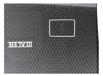
**Fig. 8.** Digital image of honeycomb structure airplane wing fragment with defective rectangle zone selected for further testing by digital solid-state transducer S10811-11of Hamamatsu Company (Japan).
