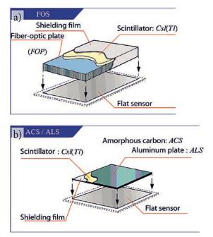
Fig. 5. Design variants of flat flaw detectors of Hamamatsu Photonics company (a) design in which image from screen to sensor is transferred by fiber-optic plate; (b) design with direct positioning of scintillation screen over sensor (CCD-matrix)
