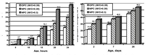
Fig. 1. Compressive strength of fine-grained concretes (C:S = 1:3) based on OPC and nanomodified Portland cement compositions
