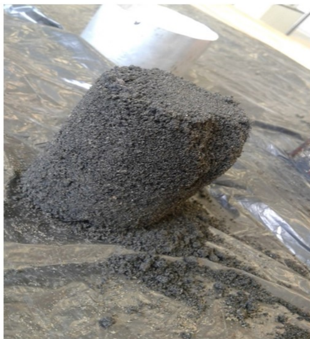
Fig. 6. Picture of test specimen obtained for Furotec 132 resin bonded + 50% Furocure CH Fast acid
