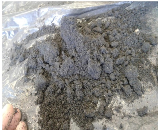
Fig. 4. Picture of crumbly mulled sand obtained for Furotec 132 resin + 70% Furocure CH Fast acid
