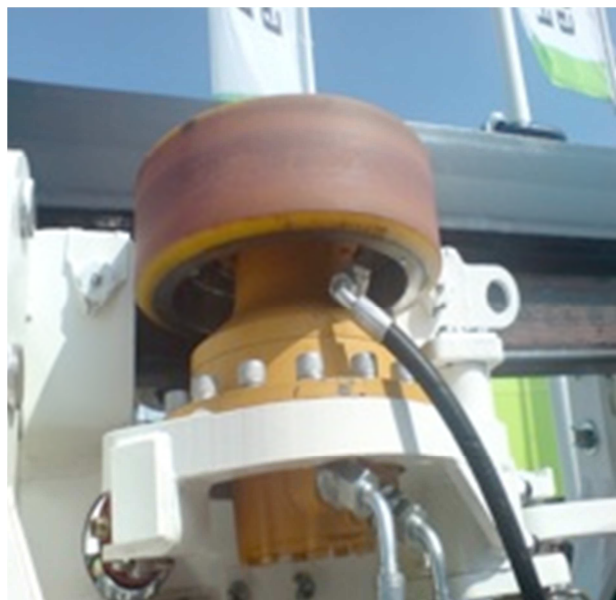
Fig.2. Friction duo “drive wheel – rail” with the corresponding force distribution in the ortogonal setup of coordinates x, y, z
