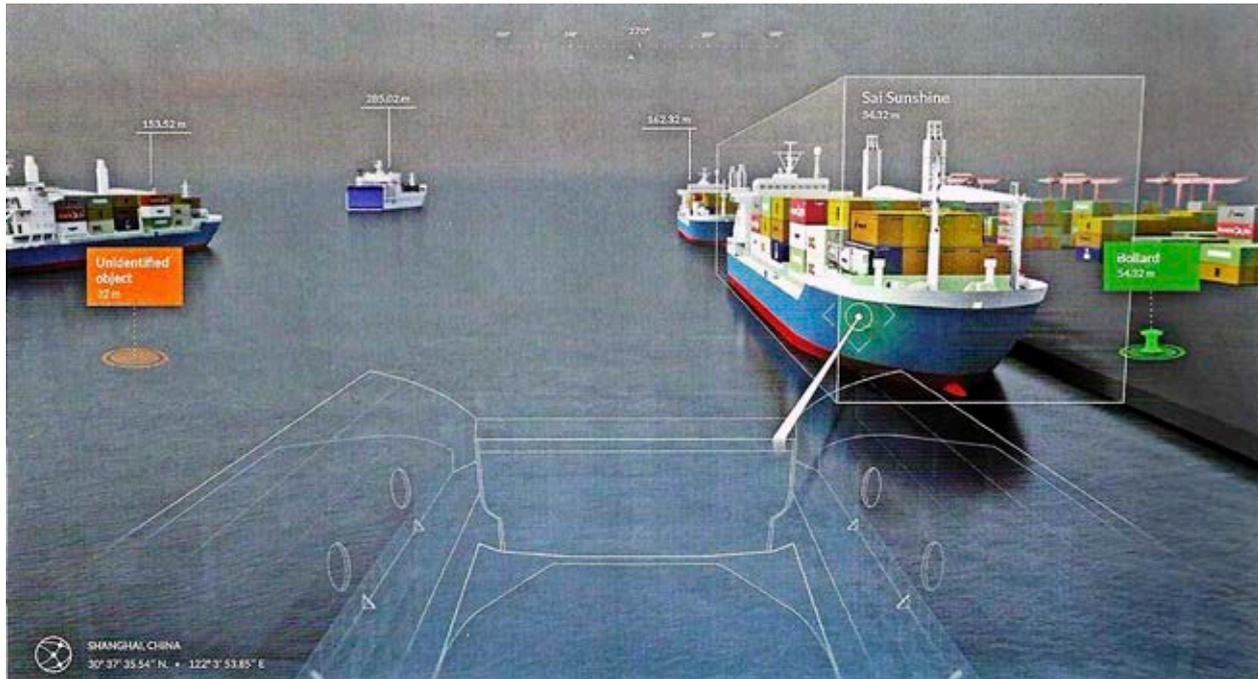
Figure 4. Rolls Royce's intelligent awareness bridge system (The Naval Architect, 2017b)
