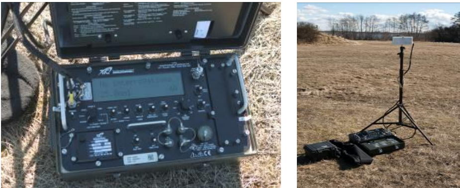
Fig. 5. Overview of the T-47G tester (left: control panel and power supply module; right: Tx/Rx antenna)
