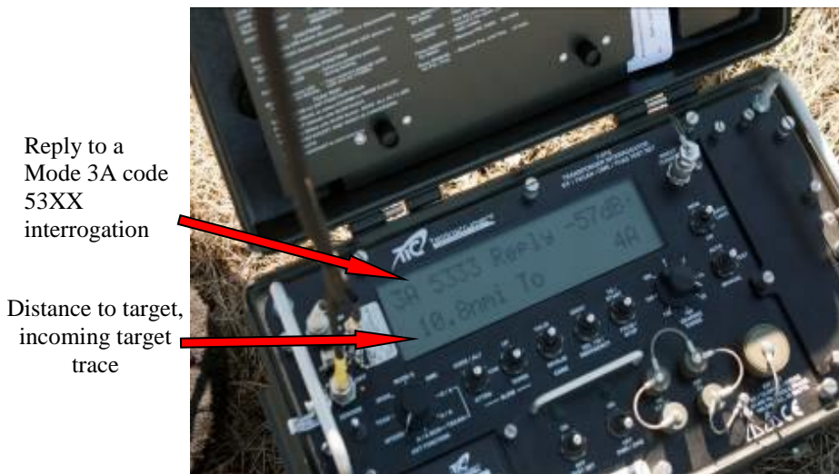
Fig. 6. Positive Mode 3/A “friend” reply to the IKZ-02P IFF interrogation – test distance to target trace: 10.8 nmi (200 hm) – incoming target trace
