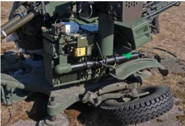
Fig. 3. Layout of the IKZ-02P IFF interrogator system components on the JODEK-SP ADGRAS TD
