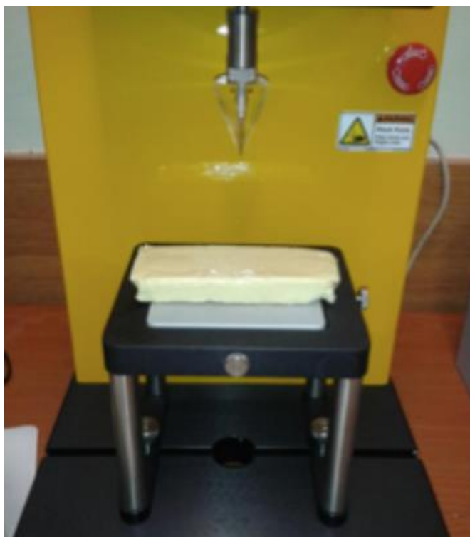
Fig. 4. Testing of the 3rd processed cheese sample using a texture analyzer.
