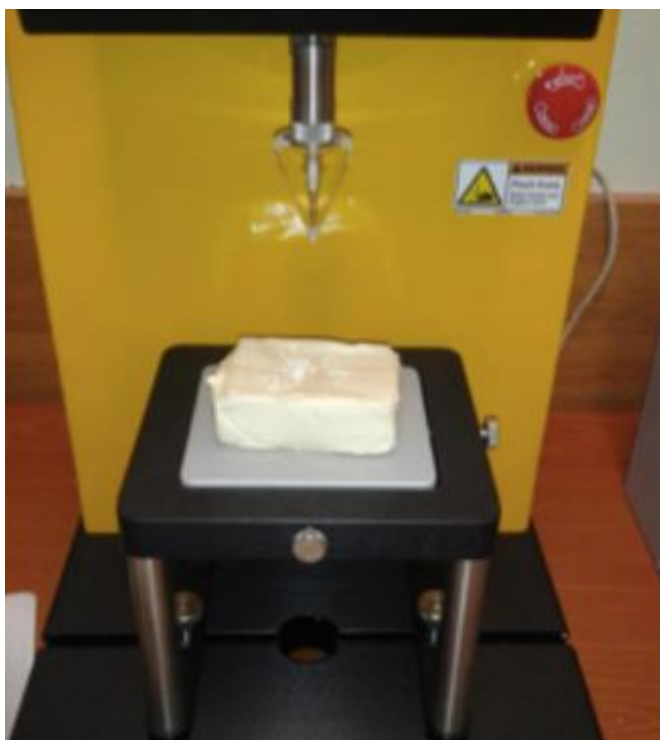
Fig. 3. Testing of the 2nd processed cheese sample using a texture analyzer.
