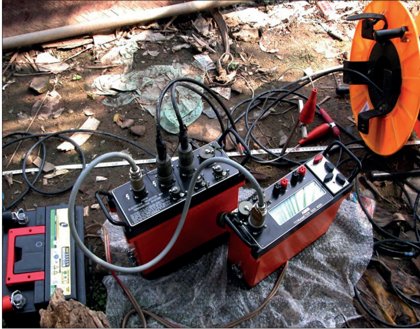
Fig. 5. Lund multi-electrode switching system connected to an SAS4000 resistivity meter of ABEM, Sweden
