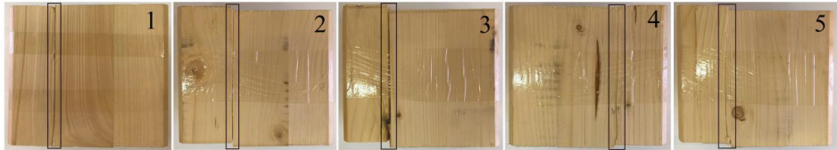
Fig. 9. Double lap shear samples after the test
