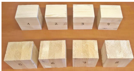
Fig. 1. Samples for the compression test
