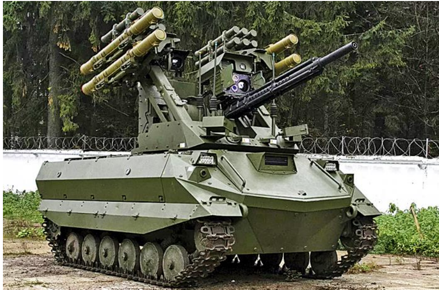
Figure 3. Russian unmanned combat platform BMRK/RROP (Boyevo mnogofunkcionalnyy robototiechnicheskiy kompleks - robot-technical combat multi-role system/Robot razvedki i ogniewoj poddierzki - reconnaissance and fire support robot Uran-9
