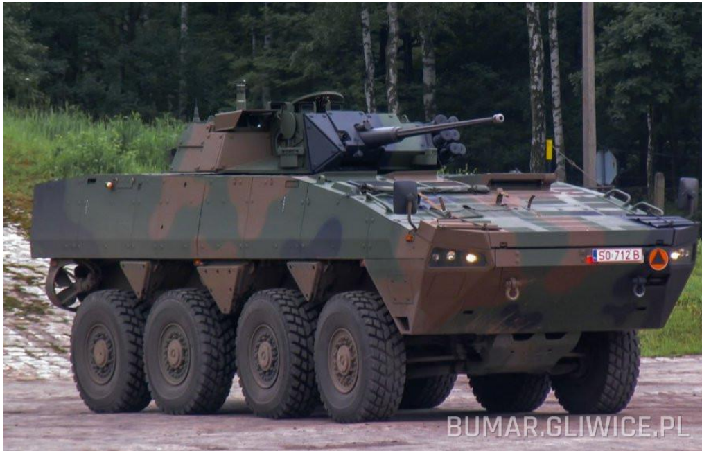
Figure 20. HITWIS turret system on KTO ROSOMAK chassis
