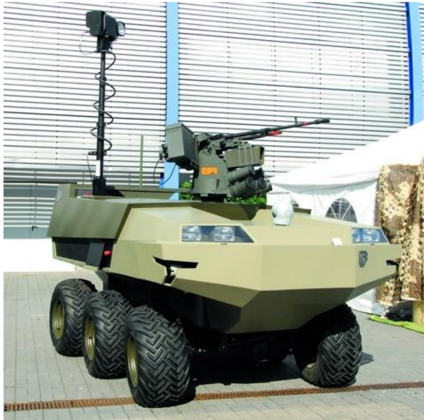
Figure 11. Polish unmanned structure LEWIATAN with unmanned turret system KOBUS from ZM Tarnów
