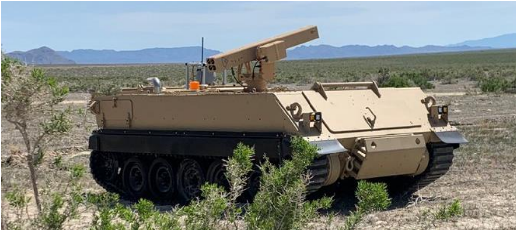
Figure 7. Modified unmanned M113 transporter with mounted Arnold Defense LAND-LGR4 remote-controlled missile launcher containing laser-guided APKWS missiles
