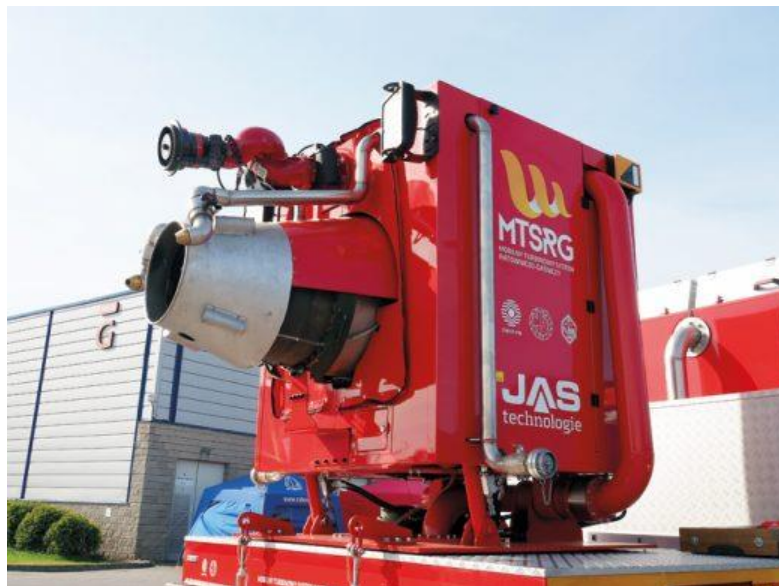
Figure 21: Firefighting device based on the use of the SO-03 jet engine of the TS 11 ISKRA aircraft
