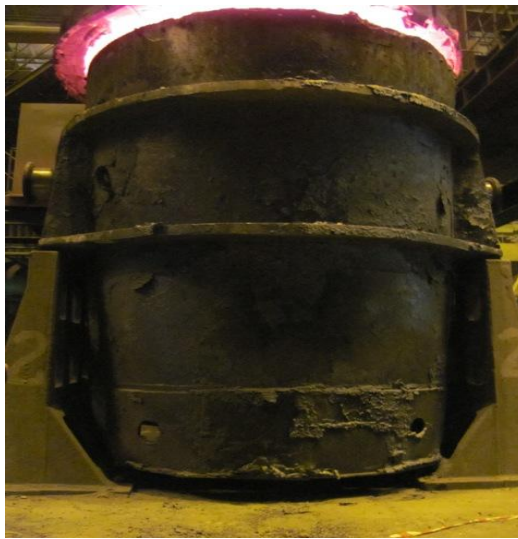
Fig. 1. Hot metal ladle in the researched company.
