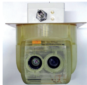
Fig. 8. The gimbal camera head with the video and thermovision camera [19]
