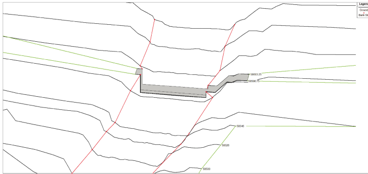
Fig. 7. Computational model of existing river bed generated in HEC–RAS
