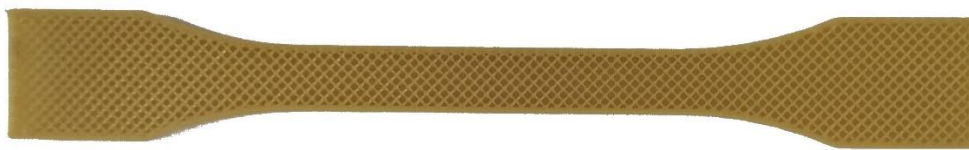
Figure 1. Cross-section of the sample with 30% grid filling
