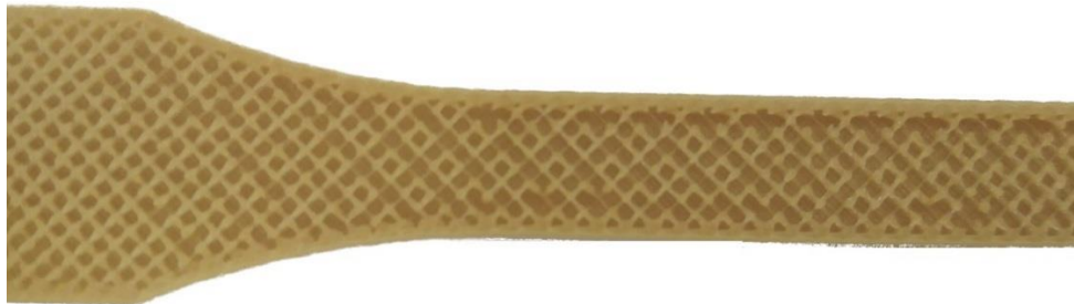
Figure 4. Printing defects - printing speed 100 \text{ mm}\cdot\text{s}^{-1}
