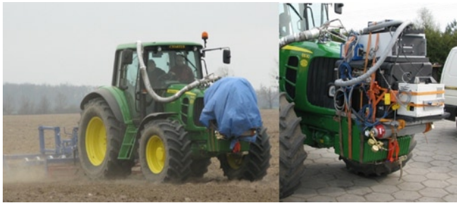
Fig. 2. The view of the tractor during the tests with the measurement equipment fitted
