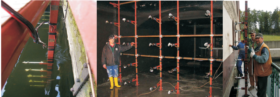
Figure 1: Current-meter measurements at the intake, in the turbine chamber and at the tailrace in Borowo ( P = 2 \times 450 kW, H = 8.10 m), Owidz ( P = 245 kW, H = 3.50 m) and Niedalino ( P = 3 \times 350 kW, H = 9.25 m) SHPs, respectively.
