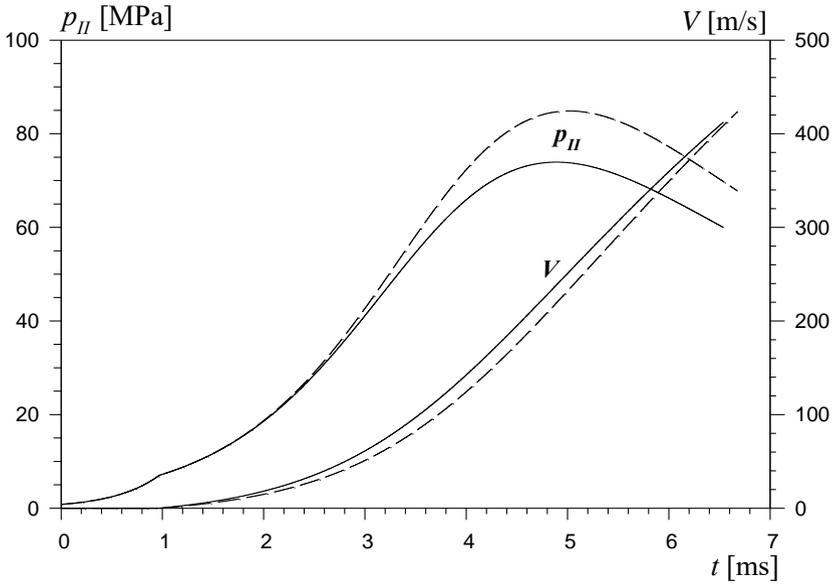
Fig. 5. The pressure  $p_{II}$  inside the barrel and projectile velocity  $V$  vs. the time  $t$ : case I – dashed line, case II – solid line
