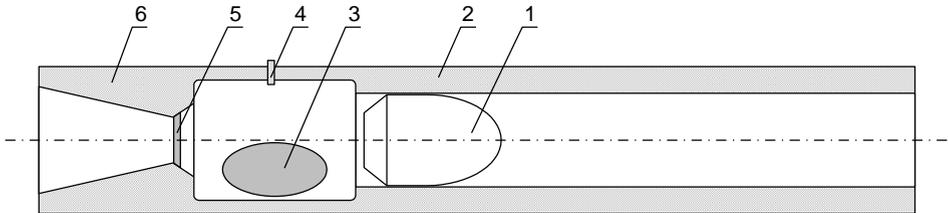
Fig. 1. Schematic of the recoilless propellant system:
