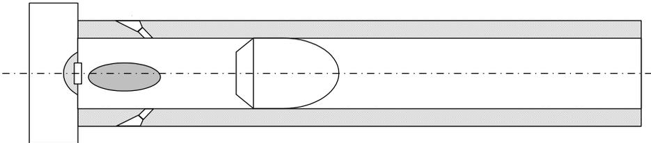
Fig. 3b. Schematic of the recoilless propellant system with not moving propellant
