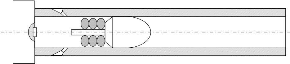
Fig. 3a. Schematic of the recoilless propellant system with the propellant connected to the projectile
