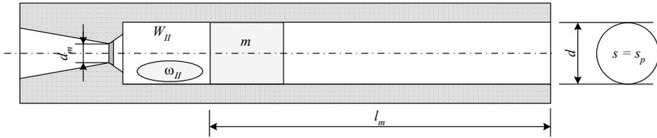
Fig. 4. Ballistic model and nomenclature of a recoilless system:
