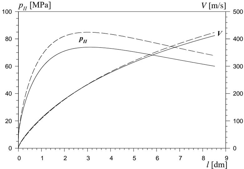
Fig. 6. The pressure  $p_{II}$  inside the barrel and the projectile velocity  $V$  vs. the projectile travel  $l$ : case I – dashed line, case II – solid line
