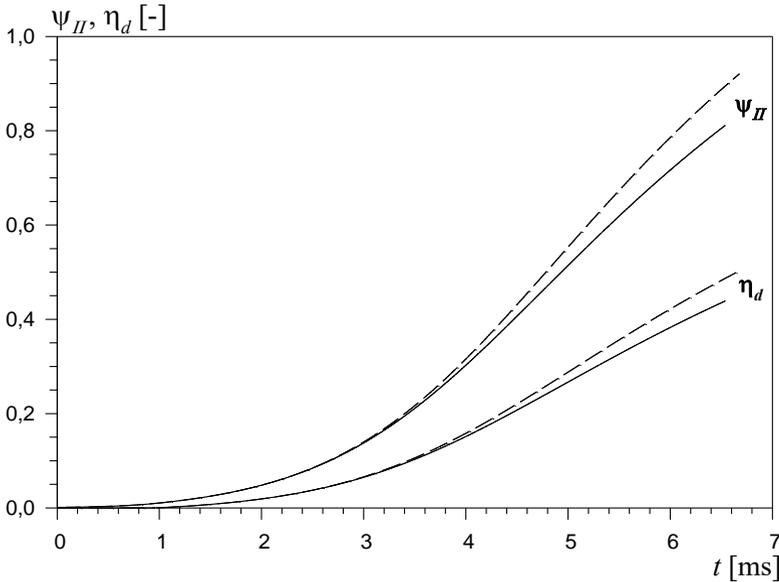
Fig. 7. Relative amount of the burned propellant  $\psi_{II}$  and the fraction of propellant  $\eta_d$ , which flew out of the barrel vs. time  $t$ : case I – dashed line, case II – solid line
