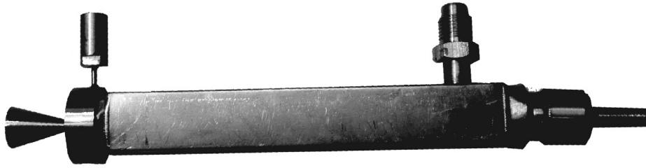
Fig. 6. Final version of the resistojet thruster
