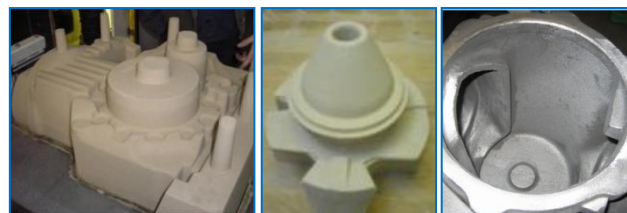
Fig. 10. Large core made on the core shooting machine (left). Small core made on the core shooting machine, addition level: 100 weight parts of sand ST55, 3.0% of GEOPOL® binder, 0.7% of GEOTEK accelerator (middle). Grey cast iron casting, the core was made from GEOPOL® CO 2 mixture (right)
