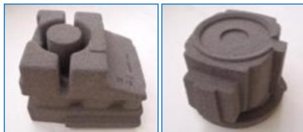
Fig. 6. Smaller cores made from 100% reclaimed sand by the GEOPOL ® technology, the self-hardening sand mixture
