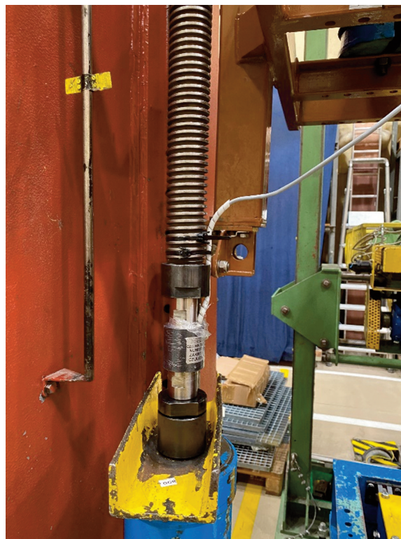
Figure 5. Lift force system screw with force transducer. (source: Landing Gear Laboratory, L-ILOT)
