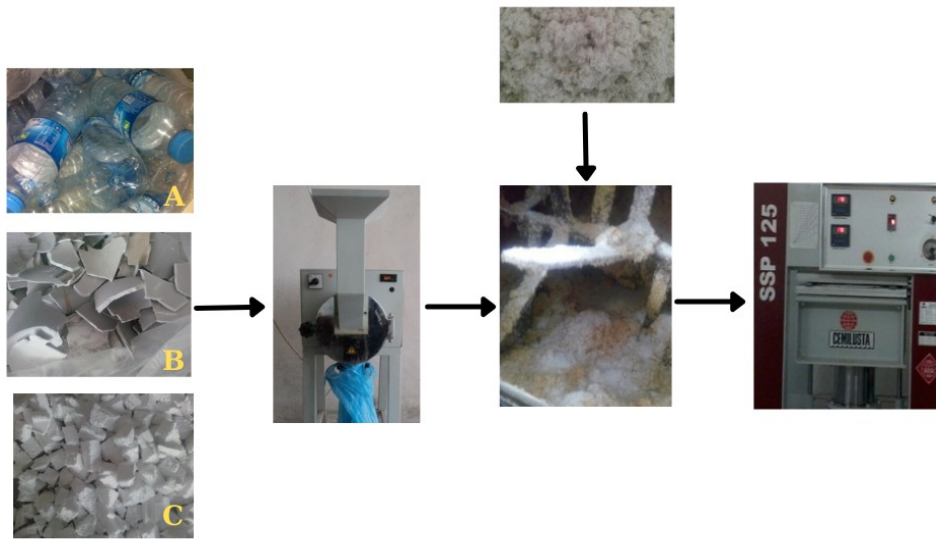
Fig. 1. Addition of waste plastics to the produced boards (A: PET wastes, B: PP wastes, C: PS wastes)
