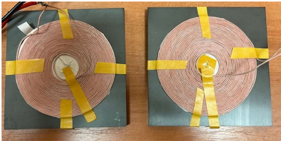
Fig. 2. Mounting manner of the windings of the tested air transformer on the ferrite plates
