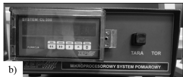
Fig. 3. Test apparatus – pin-on-disc station and force measurement system: a) Pin-on-disc station, b) Friction force measurement system
