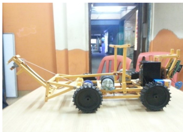
Pictures of the bridge carrying robot using ZigBee
